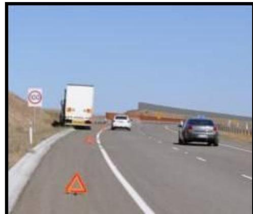
Triangles should be placed at 2.5 x Speed limit in an 80km/h or above speed zone.
