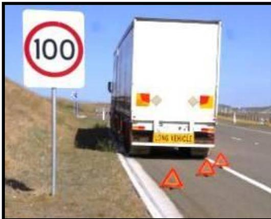
Advance warning should be appropriately spaced and not encroach into a running lane.
