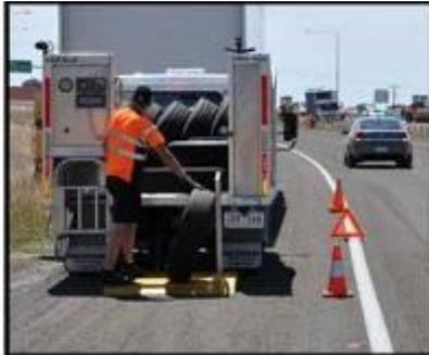
Parking parallel to traffic may be required when access to the rear of the vehicle is essential.
